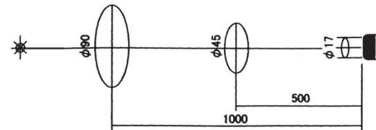
The above measuring diameter is defined as an area which allows capture of more than 90% of energy.
