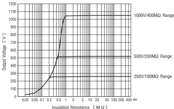
● Principle of Insulation Resistance Measurement
