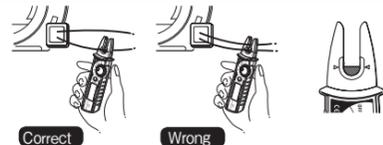
Place the center of the measured conductor lower than the triangle mark indicated on the fork shaped sensor. (shaded part in the figure)
