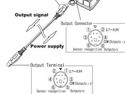
\* Pin assignment at the connecting terminal of measuring instrument (MODEL6300, KEW5010 / 5020) is symmetrical to above figure.
