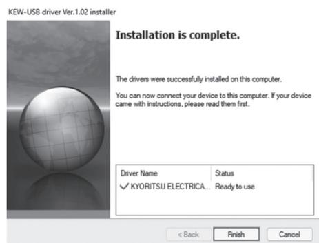
The USB driver has been successfully installed. Power on KEW6315 first, and then connect to you PC.
