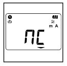
4. Can make measurement right after powering on the instrument. When nc (non-connect) is displayed on the LCD, a sensor is not connected to the appropriate channel; or the connection is incorrect. Step2: Confirmation and change of set value
