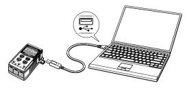
(2) Connect the other end of USB cable to the USB terminal on the right side of this instrument.
