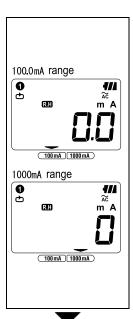
4. Press the button to switch the measurement ranges at each channel. The Range hold function is activated when the RH mark is displayed on the LCD.
