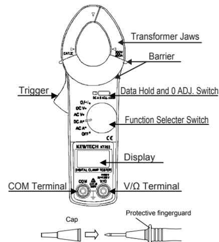
Protective fingerguard (Barrier) : It is a part providing protection against electrical shock and ensuring the minimum required air and creepage distances.
