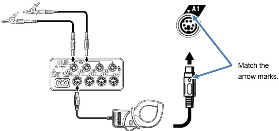
Number of Voltage test leads and Clamp sensors to be used will be different depending on the wiring configuration under test. For further details, refer to “*Wiring diagrams*” (P.50) in this manual.
