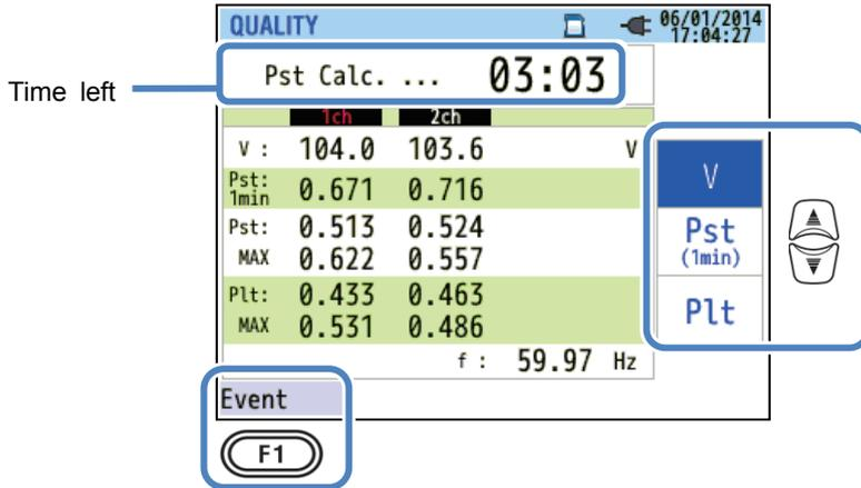
If variable loads, such as arc furnace, are connected, voltages may vary and cause changes in illumination levels. Such phenomenon is called as “voltage flicker” and its severity level is indicated by “Pst” and “Plt”.
