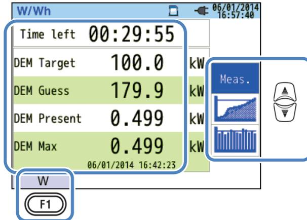
The demand is the average powers recorded over a certain period. When the estimated value exceeds the target value during demand measurements, the warning buzzer sounds at the inspection cycles.
