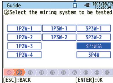
(2) Select the wiring system to be measured.
