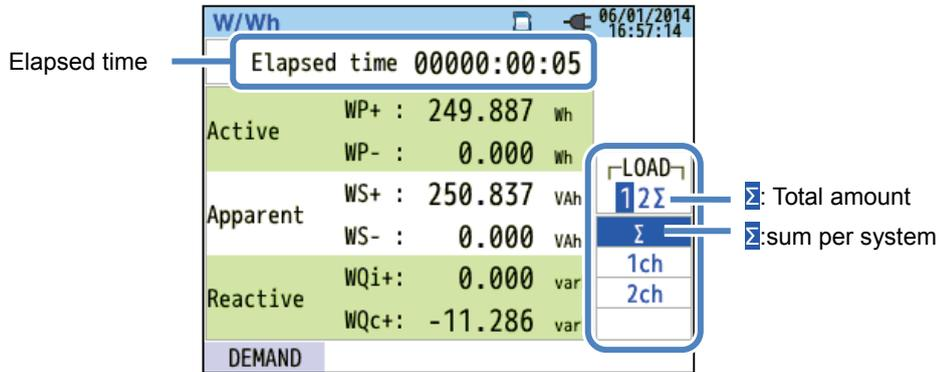
Power used in the certain period is displayed as integral power consumption. Integral power consumption is used to calculate electricity tariffs or to control the power consumption.
