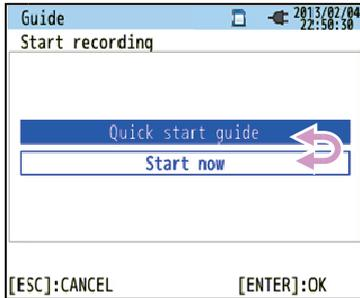
Press the **Cursor** Key to move the **blue highlight**, showing the item is being selected, over the items in blue letters. In the screen to the left is the Recording start screen. Press the **Cursor** Key and move the blue highlight on the desirable recording method, and press the **ENTER** Key to confirm the selection. To quit the start guide, press the **ESC** Key.
