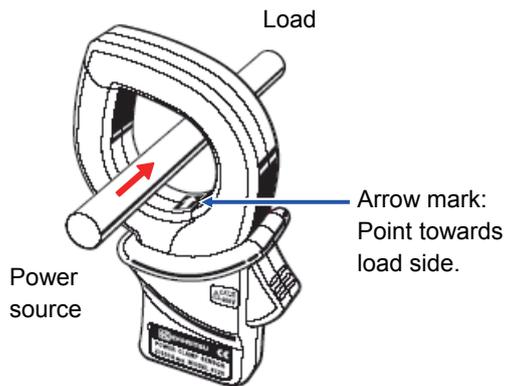
Reverse clamping switches the symbols (+/-) for active power (P).
