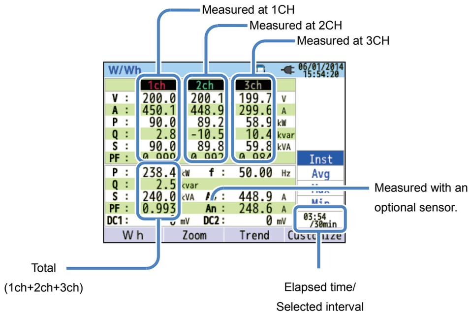
Multiple measured values can be displayed on one screen. The displayed items can be changed by pressing the corresponding keys.
