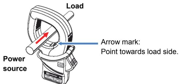
\* Reverse clamping switches the symbols (+/-) for active power (P).
