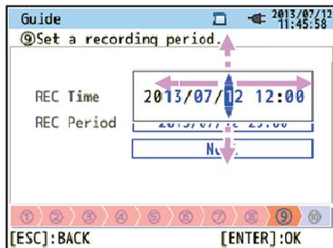
To alter the numbers such as **Date/ Time**, move the blue highlight over digits with the right and left **Cursor** Keys and alter the number with the up and down **Cursor** Keys. In the screen to the left, the tenth place of the day is being selected. The number can be increased or decreased by 1 with the up/ down **Cursor** Keys. Press the **ENTER** Key to confirm the selection, or press the **ESC** Key to return to the previous screen and cancel the changes.
