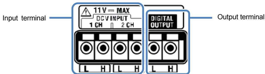
Ensure that the wires are connected to proper terminals.
