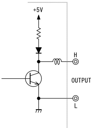
Output format : Open collector output
