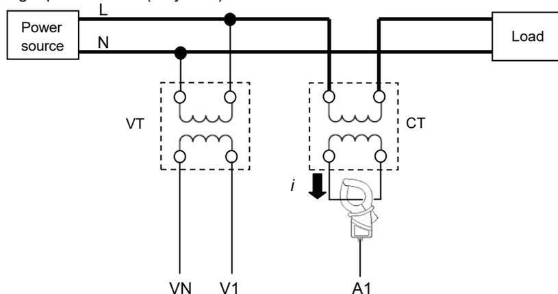
When rating of the secondary side of CT is 5A, use of Clamp sensor 8128/8135 (50A type) and testing at 5A Range is recommended.
