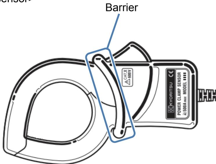
Protective fingerguard and barrier is a mechanical safety part and provides protection against electrical shock and ensuring the minimum required air and creepage distances. Keep your fingers and hands behind the protective fingerguard and barrier during a measurement.
