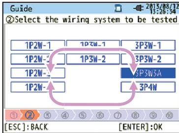
If the display of the **selectable items** is similar to the one shown to the left, then the up, down, right and left **Cursor** Keys can be used. Use the **Cursor** Keys to select the proper wiring system and press the **ENTER** Key to confirm the selection. To return to the previous screen and cancel the changes, press the **ESC** Key.
