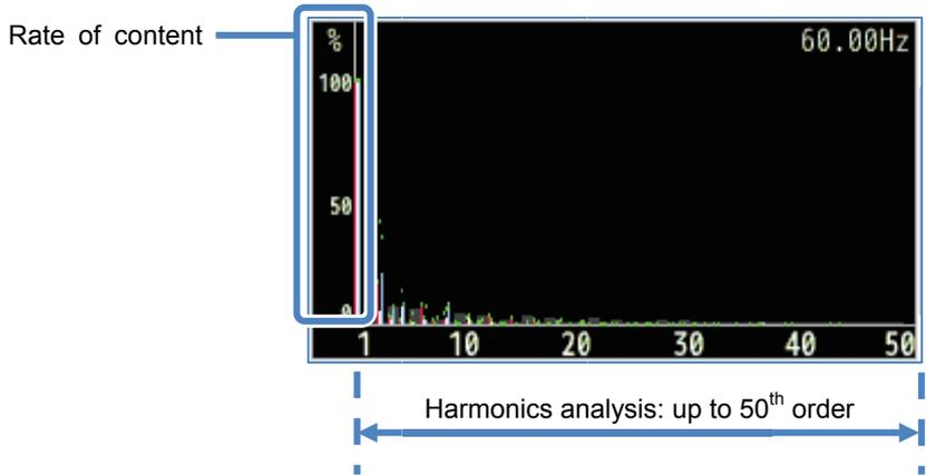
In the above example, "Linear" and "full-scale" are selected. In this case, the upper limit of the rate of content is "100%" and all harmonics, 1<sup>st</sup> to 50<sup>th</sup>, are displayed on one screen.
