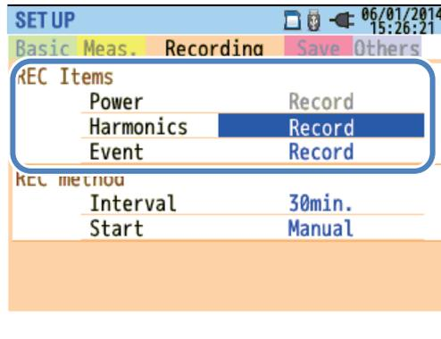
The possible recording time on SD cards or the internal memory varies depending on the number of the recorded items and the preset intervals. Select “Do not record” for the items which are not necessary to be recorded to secure a longer recording time. The details are described in **“Possible recording time”(P. 76)**.
