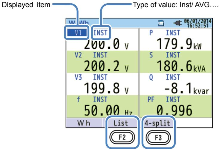
Select 4 or 8 values and display the values on one screen. The displayed text will be enlarged so it is easy to see.
