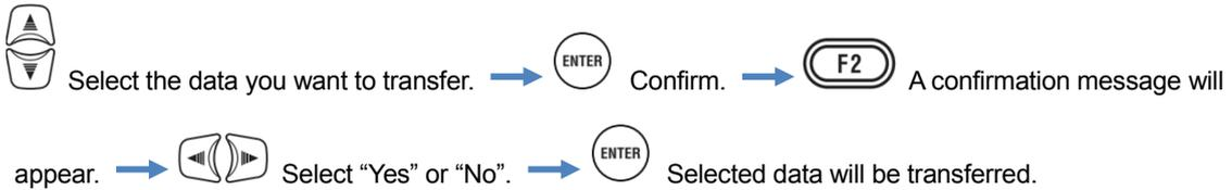
A check mark “
