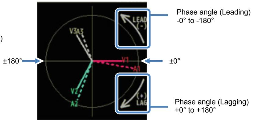
The circle (solid line) represents the max values at V and A Ranges, and the line length represents rms voltage and current values. The angle between the lines represents phase relation with reference to V1. For 3P3W3A/3P4W, unbalance ratio is also displayed. While the measured voltages and currents are balanced, the following vectors will be displayed.
