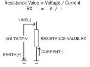
Terminal connection of insulation resistance test In case of testing insulation of insulated wire and cable against the earth at direct current, connecting – pole of power to cable conductor, + to the earth obtains smaller measuring value, compared with connecting the other way round. This connecting method is generally acknowledged relevant to detect defective insulation.
