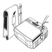
Pass the strap belt down through the side panel of the main body from the top, and up through the slots of the probe case from the bottom.
