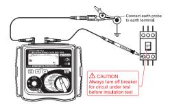
(§) With the test probe still connected to the circuit under test, release the test button to discharge capacitance in the circuit after measurement.
