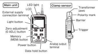
Barrier: It is a part providing protection against electrical shock and ensuring the minimum required air and creepage distances.
