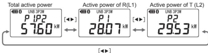
A long press of mode button clears measured results and the screen returns to the initial screen.
