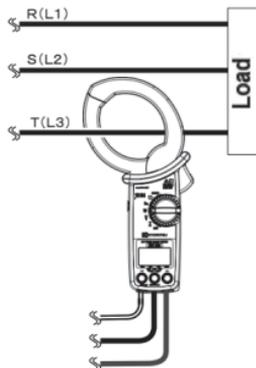
Press the item switching button [▶] after making connection, the LCD shows active power of T(L3) phase. Pressing mode button switches the indications between active power and RMS voltage/ current values of T(L3) phase.
