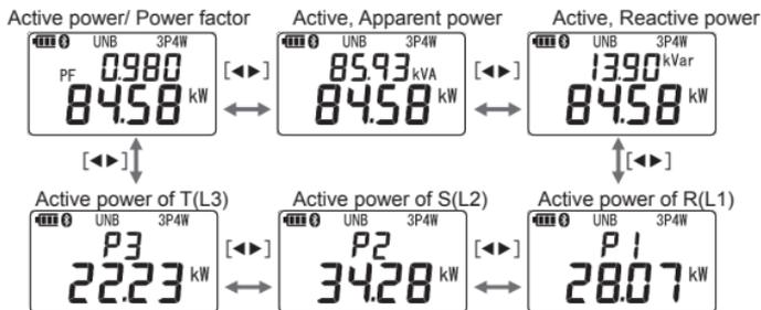
A long press of mode button clears measured results and the screen returns to the initial measurement setting screen.
