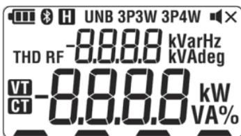
When setting the function switch to any position other than "OFF", KEW 2060BT gets started and all the LCD segments are displayed for 1 sec. Confirm that there're no chips of segments.
