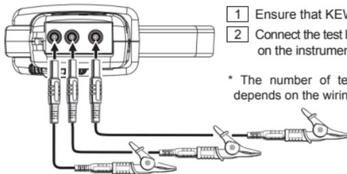
Connect the test leads per the following procedures.
