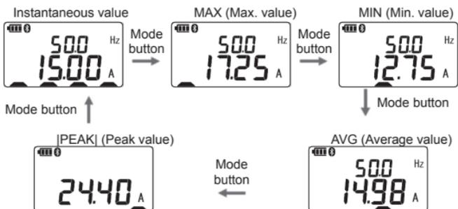
Range is fixed while the LCD is showing MAX, MIN, AVG, or |PEAK|. The auto-ranging function is reactivated when switching the display to instantaneous value.
