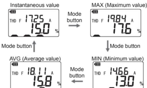
Range is fixed while the LCD is showing MAX, MIN, or AVG. The auto-ranging function is reactivated when switching the display to instantaneous value.
