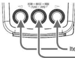
Press the item switching button [◀▶] to toggle the displayed items and confirm the desired item with the mode button. Alter the values of each item with the item switching button [◀▶], and then press the mode button again to confirm the change. The display returns to the selection screen.
