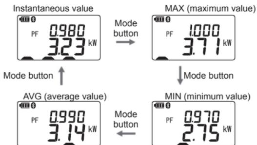
Range is fixed while the LCD is showing MAX, MIN, or AVG. The auto-ranging function is reactivated when switching the display to instantaneous value.
