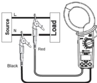
When the unit shown in the LCD is "A", it means the screen is "current harmonics measurement screen". Hold down (long press) the Item switching button [▶] to switch the unit to "V".
