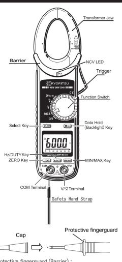
Protective fingerguard (Barrier) : It is a part providing protection against electrical shock and ensuring the minimum required air and creepage distances.
