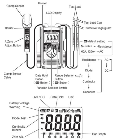
**Clamp Sensor** : Pick up current flowing through the conductor.
