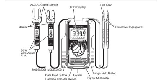
Barrier Protective fingerguard : It is a part providing protection against electrical shock and ensuring the minimum required air and creepage distances.
