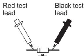
Figure 2 Reverse-bias Diode Test
