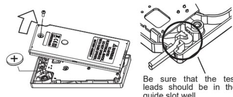
Be sure that the test leads should be in the guide slot well.
