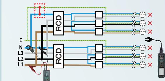
If N and E are connected each other in the circuit downstream to KEW 8343, KEW 4506 cannot work properly.
