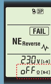
KEW 4506 has a mode which can detect the wiring connection avoiding any RCD tripping. \*resistance measurement OFF
