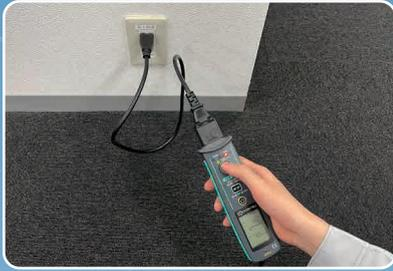
Easy measurement by simply plugging into a socket outlet and pressing the test button.
