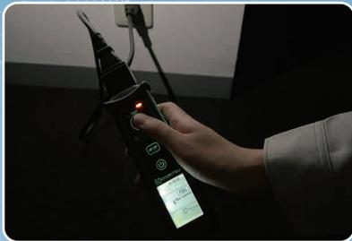
LCD backlight automatically turns on at the dark place.
