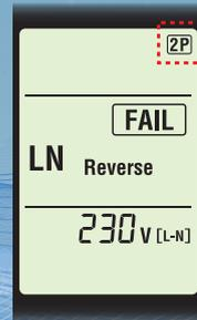
Wiring check for 2P(no earth) outlet is also available by selecting the 2P setting. \*2P conversion adapter which is required to connect with 2P outlet isn't supplied.
