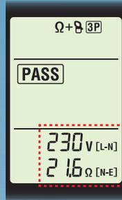
L-N voltage and N-E resistance at TT system can be displayed.
