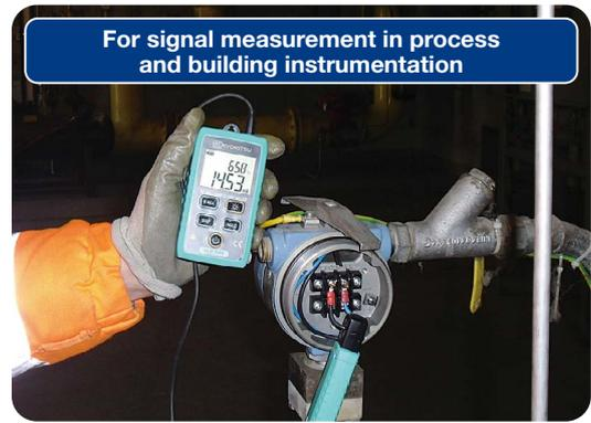
For signal measurement in process and building instrumentation
