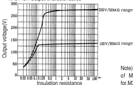
Note) For the output characteristics of M3148A, see the left graph for M3145A.
