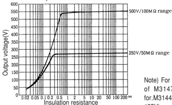
Note) For the output characteristics of M3147A, see the left graph for M3144A (at 500V) and 3145A (at 125V).
