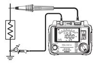
▲ Caution Always turn off the Breaker for the circuit under test.
