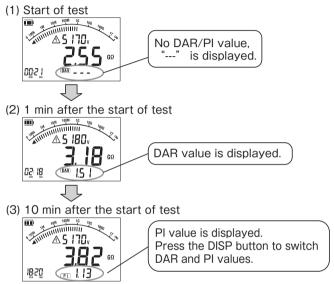
5. How to review the measured DAR/ PI values Press the DISP button after a measurement. The measured results are then displayed in the following sequence. If a measurement ends earlier than the intervals described in below (2), (3) or (4), nothing will be displayed and returns to the initial state (1).
