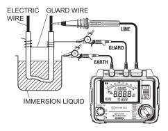
\* It is possible to move out the surface leakage resistance of the insulation and measure only the volume resistance by using the Guard terminal. This is helpful when performing tests in humid air.
