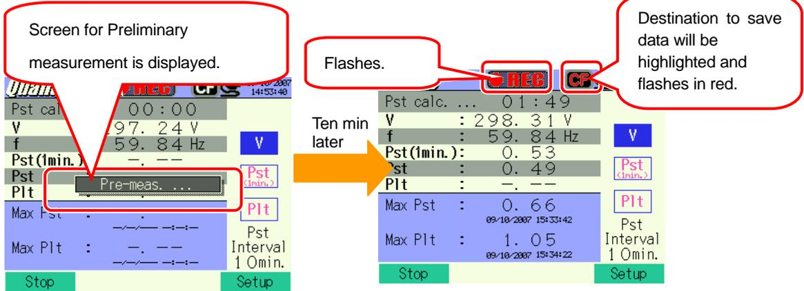
Setting cannot be done during a data saving. Press the **F4** Key to check settings.
