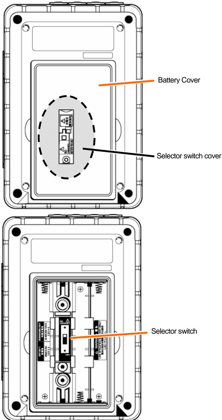
\* Set the Selector Switch to either "DRY BATTERY" (alkaline) or "RECHARGEABLE BATTERY" (Ni-MH) position depending on the battery you use.
