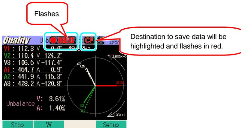
Settings cannot be done during a data saving. Press the **F4** Key to check the settings.
