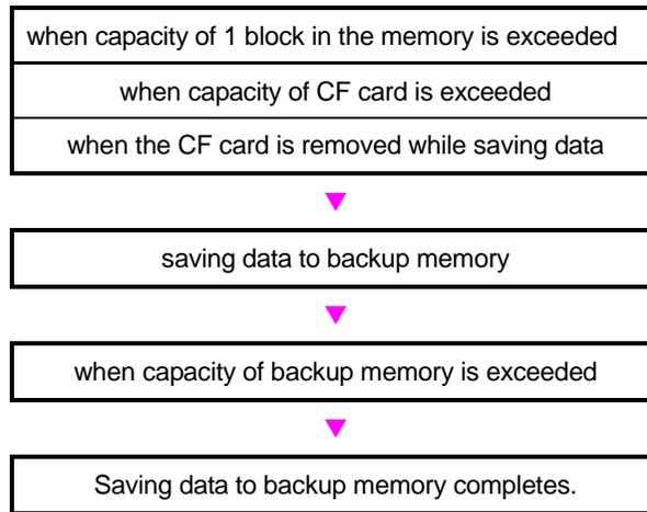
Data saved in the backup memory is kept after powering off the instrument, however, it will be overwritten every time starting backup function.
