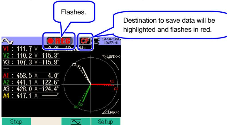
No setting change can be made during data saving . Press the **F4** Key to check the settings.
