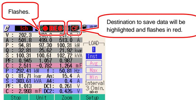
Setting cannot be done during a data saving. Press the **F4** Key to check settings.
