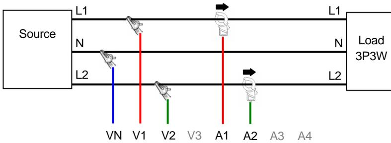
6. "1P3W x 2" Wiring method for single-phase 3-wire (2ch)
