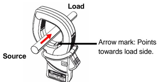
\* Reverse clamping switches the symbols (+/-) for active power [P].
