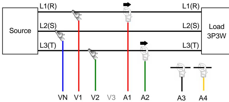
11. "3P3W 3A" Wiring method for three-phase 3-wire + 3-current
