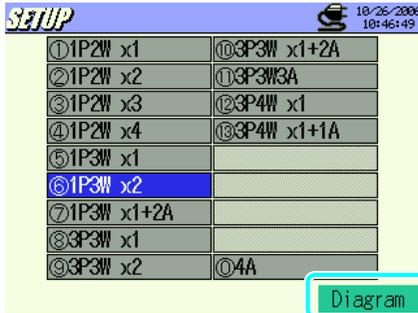
Press the **F4** Key to display the connection diagram for the selected wiring configuration.
