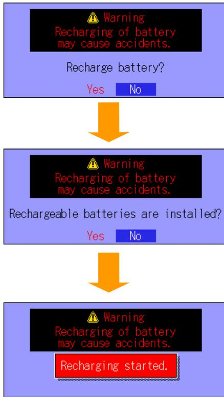
Battery charge starts and the screen returns to normal.
