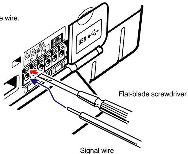
Connect wires to the proper terminals.
