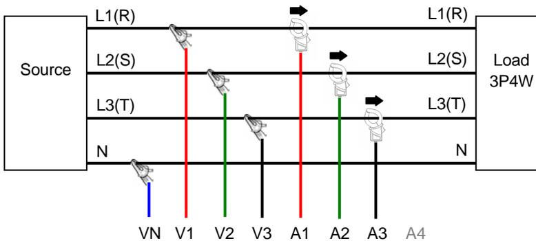
13. "3P4W x1 +1A" Wiring method for three-phase 4-wire (1ch) + 1-current
