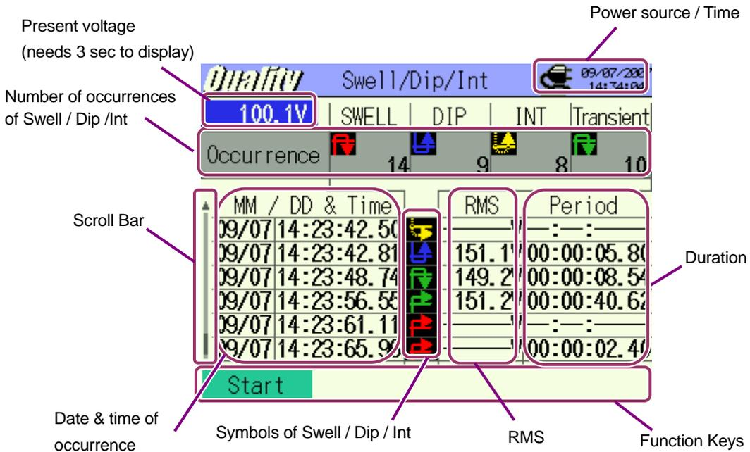
\* At Swell measurement, max RMS (voltages in duration period) is displayed and at Dip & Int measurements, min RMS is displayed respectively.
