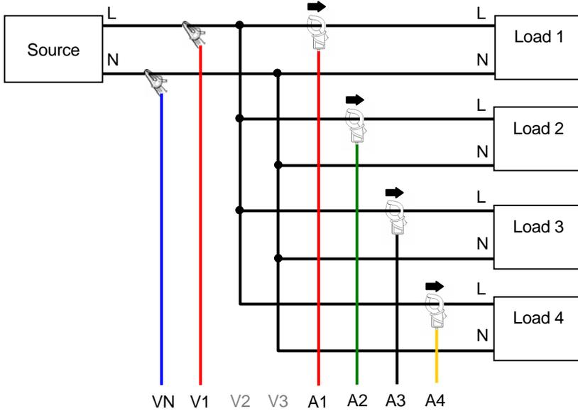
5. "1P3W x 1" Wiring method for single-phase 3-wire (1ch)
