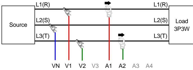
9. "3P3W x2ch" Wiring method for three-phase 3-wire (2ch)
