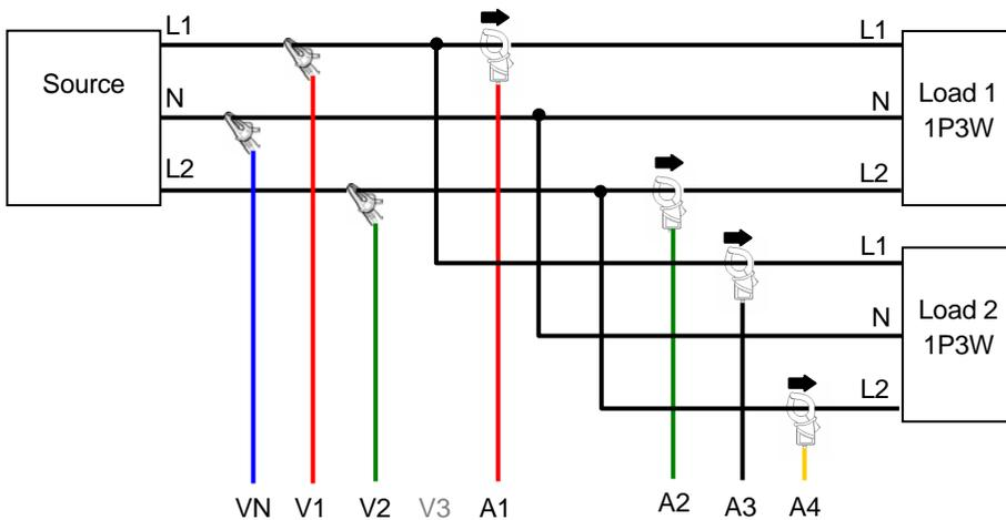
7. "1P3W x1 +2A" Wiring method for single-phase 3-wire (1ch) + 2-current
