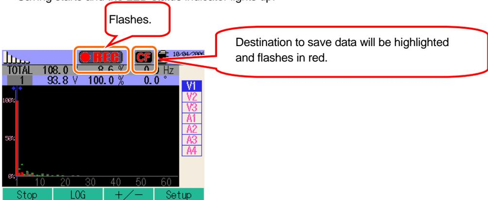
No setting change can be made during data saving . Press the **F4** Key to check the settings. The channels with "OFF" setting aren't displayed.
