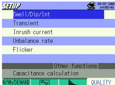
Access to “QUALITY” from Measurement Setting Tab, and press the **▲▼** **Cursor** Keys and select : Swell / Dip / Int, Transient, Inrush current, Unbalance rate, Capacitance calculation and Flicker measurement\*.
