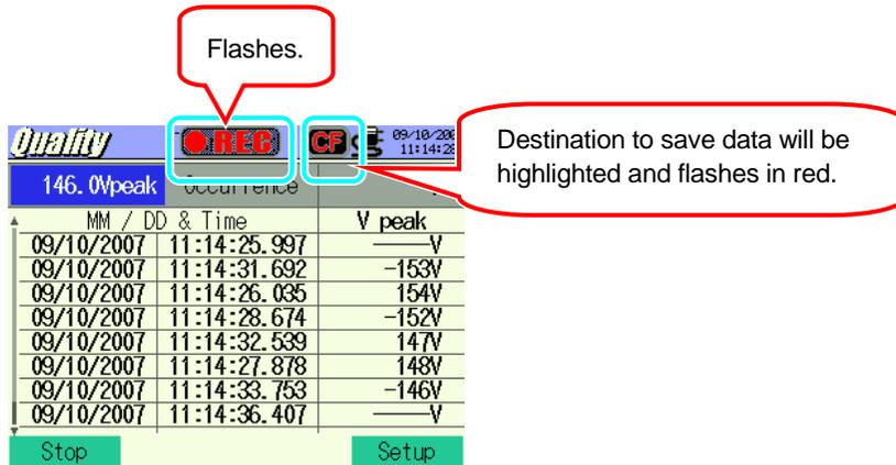
No setting change can be made during data saving. Press the **F4** Key to check the settings.
