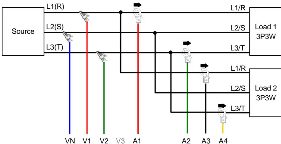
10. "3P3W x1 +2A" Wiring method for three-phase 3-wire (1ch) + 2-current
