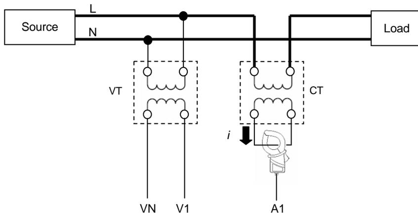
When rating of the secondary side of CT is 5A, use of Clamp sensor 8128 (50A type) and testing at 5A Range is recommended.
