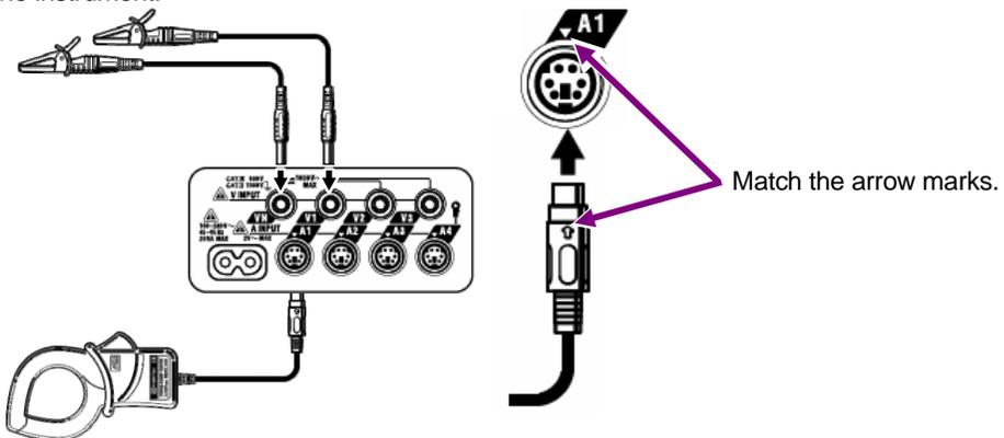
\* Number of Voltage test leads and Clamp sensors to be used depends on the wiring configuration under test. For further details, refer to “5.2 Basic Wiring Configuration” in this manual.
