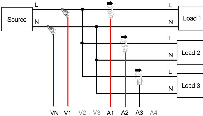
4. "1P2W x 4" Wiring method for single-phase 2-wire (4ch)
