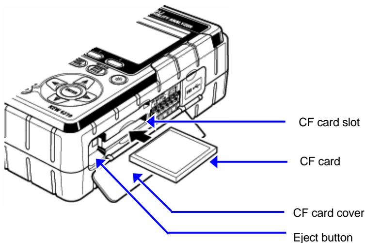
The instrument automatically detects the CF card when the card is inserted.
