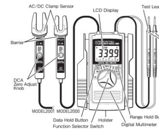
Barrier : It is a part providing protection against electrical shock and ensuring the minimum required air and creepage distances.
