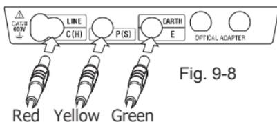
Use MODEL7228A test leads for measurement.
