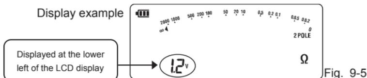
Make sure that the voltage is less than 10 V. When the display reads 10 V or more, a warning LED as shown below lights up. (The warning LED lights up at 5 V or more for an earth voltage of 400 Hz.)
