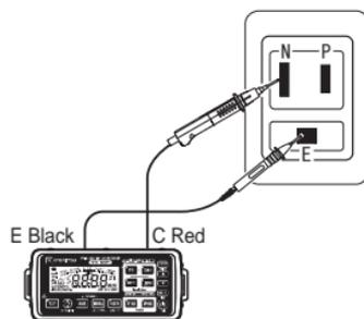
Connection using socket outlet
