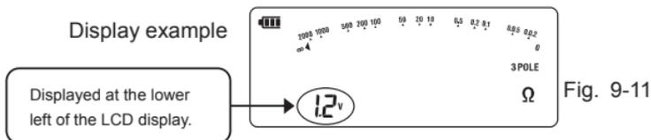
Make sure that the voltage is less than 10 V. When the display reads 10 V or more, the warning LED as shown below lights up. (The warning LED lights up at 5 V or more for an earth voltage of 400 Hz.)
