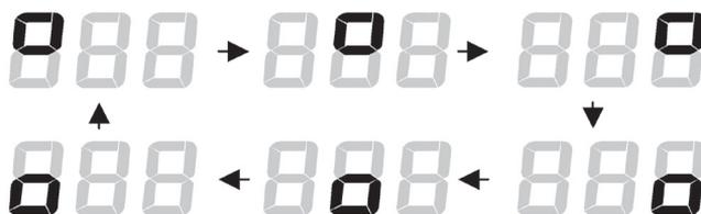
If the external earth probe is badly connected, the following symbol will be shown on the LCD and the measurement will be stopped.
