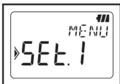
2. Press the
