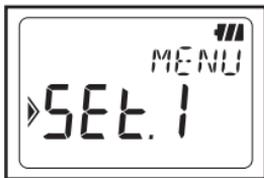
2. Press the button while instrument is on to enter into Menu mode.
