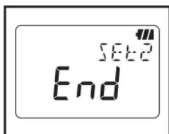
9. Now Setting 2 is completed; "End" is displayed on the LCD. Press the
