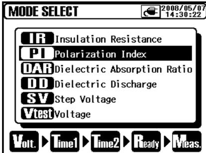
Move the cursor with the **UP/ DOWN Key** or **Shuttle Switch**, and confirm the mode with the **ENTER Key**.
