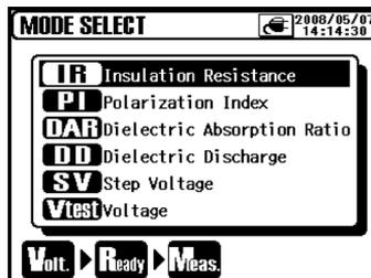
The instrument remembers the previous selected mode, and starts with the mode next time it is powered on.
