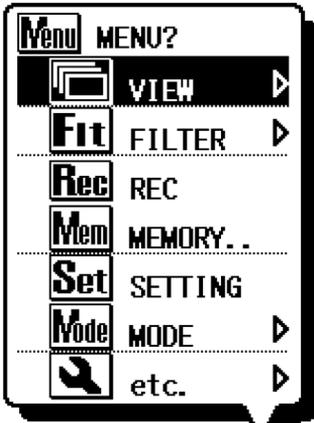
Move the cursor with the **UP/DOWN Keys** or **Shuttle Switch**, and confirm the selection with the **ENTER Key**. Pressing the **ESC Key** while the Menu is being displayed closes the Menu Window.
