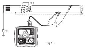
Method of Impedance test between Line and Line and Prospective Short Circuited Current test
