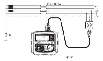
The maximum value of Zs for this example is  $2.1\Omega(16amp~gG$  fuse,0.4 seconds).The loop tester reads  $1.14\Omega$  and consequently the condition Zs $\leq$ Uo / Ia is met.
