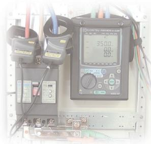
Load current detection type clamp sensors provide superior characteristic in phase for the use of power meter
