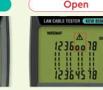
Open circuit is detected on Pins 4 and 5.
